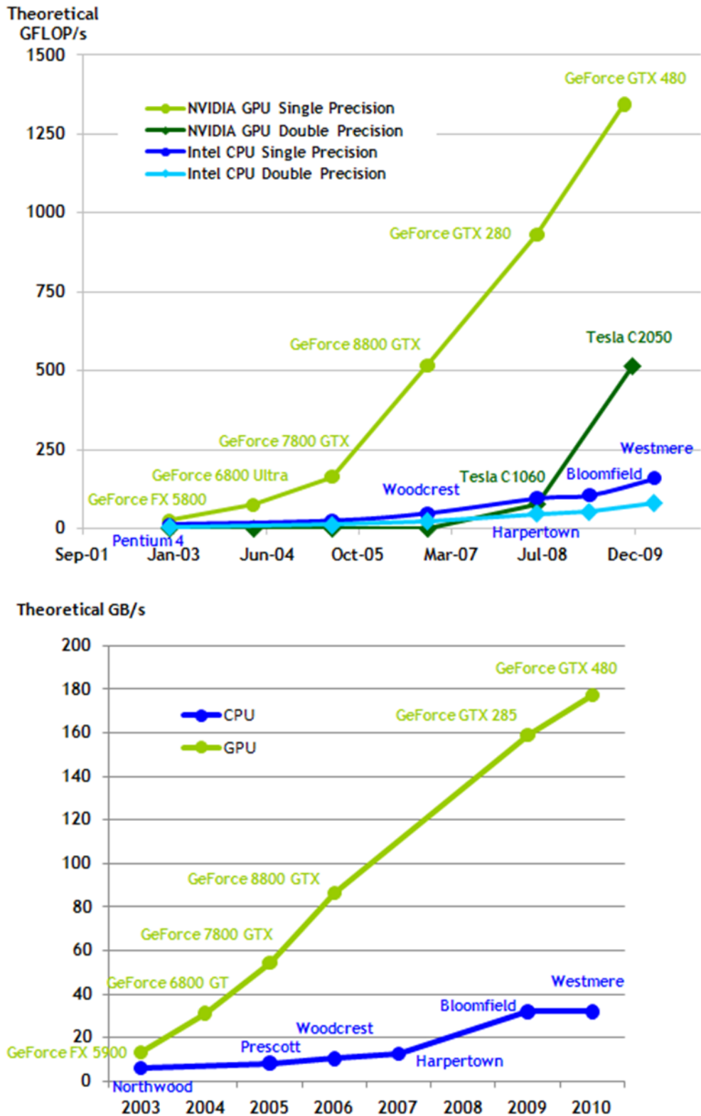
Figure 1-1. Floating-Point Operations per Second and Memory Bandwidth for the CPU and GPU
